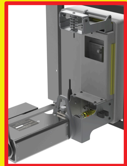
MDU WITH ATTACHED TAA PROPERLY ENGAGED WITH DRIVE RINGS AND LOCKING PIN, READY FOR SDB AND HHC COMMUNICATION CORDS
