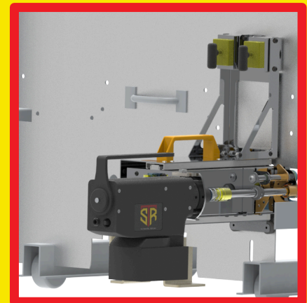
MDU WITH ATTACHED TAA PROPERLY ENGAGED WITH DRIVE RINGS AND LOCKING PIN, READY FOR SDB AND HHC COMMUNICATION CORDS
