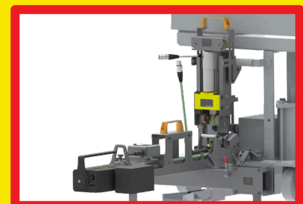
MDU PROPERLY ENGAGED WITH DRIVE RINGS AND LOCKING PIN, READY FOR SDB AND HHC COMMUNICATION CORDS
