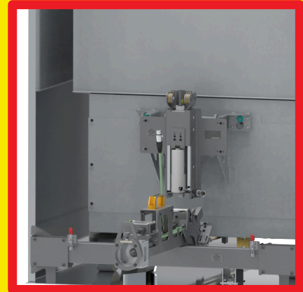
INTERLOCK MANIPULATOR SUSPENDED FROM CUBICLE KIT AND SMART DRIVE BRACKET SECURED IN PLACE - READY FOR XLR CABLE CONNECTION
