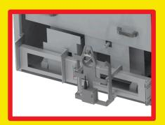
SDB SUSPENDED FROM SPANNER BAR AND ALIGNED WITH RACKING PORT
