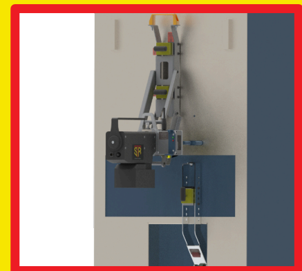
MDU WITH ATTACHED TAA ENGAGED WITH DRIVE RINGS AND LOCKING PIN, READY FOR SDB AND HHC COMMUNICATION CORDS
