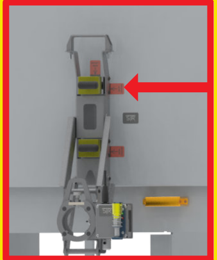
SDB PLACED AGAINST CUBICLE FACE, USING INDICATORS TO CONFIRM ALIGNMENT
